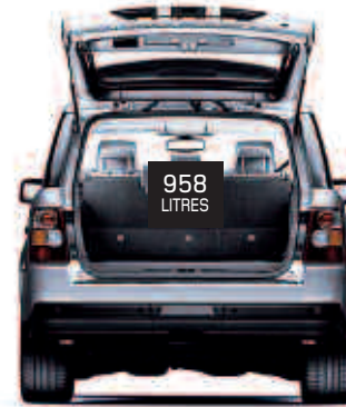
Luggage Capacity Rear seats upright Height 943mm Width 1,221mm Length at floor 991mm Loadspace volume 958 litres Loadspace width between arches 1,120mm
